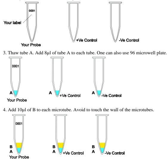
TIP: you can mix  $8\mu$ l of A + 10 $\mu$ l of B together in one tube (it will be a total volume of 180 $\mu$ l for 10 reactions). From this one can take 18 $\mu$ l and distribute in each tube. In this way one can save the hardware and time.
