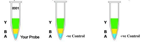
TIP: Add  $7\mu l A + 10\mu l B + 1\mu l Y = 18\mu l$  per reaction. In case you want to run 10 reactions i.e. you need total  $180\mu l$ , therefore you should mix  $70\mu l$  of  $A + 100\mu l$  of  $B + 10\mu l$  of  $Y = 180\mu l$  from which you can take  $18\mu l$  and add to each tube. This way you save time and hardware.
