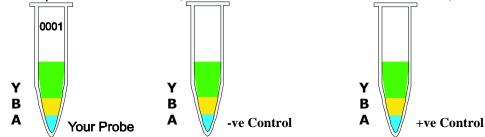
TIP: Add  $7\mu l\ A + 10\mu l\ B + 1\mu l\ Y = 18\mu l\ per\ reaction.$  In case you want to run 10 reactions i.e. you need total 180 $\mu l$ , therefore you should mix  $70\mu l$  of  $A + 100\mu l$  of  $B + 10\mu l$  of  $Y = 180\mu l$  from which you can take 18 $\mu l$  and add to each tube. This way you save time and hardware.
