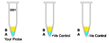
TIP: you can mix  $8\mu l$  of  $A+10\mu l$  of B together in one tube (it will be a total volume of  $180\mu l$  for 10 reactions). From this one can take  $18\mu l$  and distribute in each tube. In this way one can save the hardware and time.
