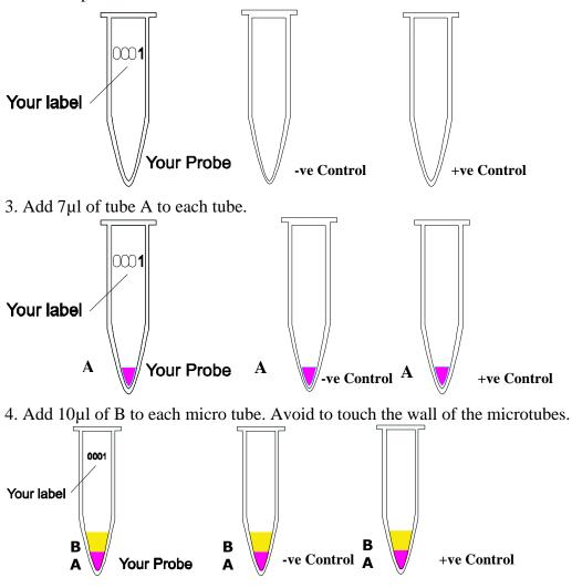
5. Add 1µl of Y to each tube (avoid to touch the wall of the microtubes).
